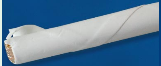
Wire with conventional PTFE tape wrap insulation can fray when stripped.
